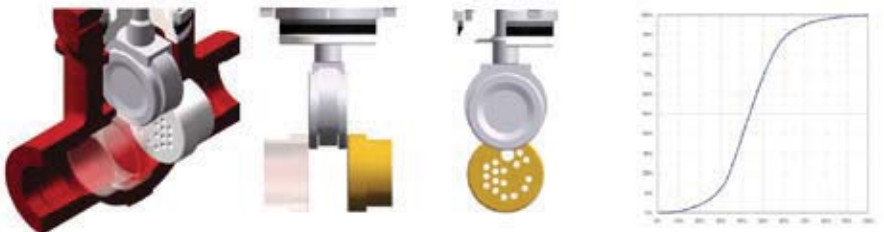
Bypass sizes according MSS SP - 45, Series A
