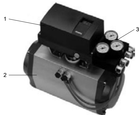
Illustration 2: Positioner mounted on a linear actuator (single-acting)
