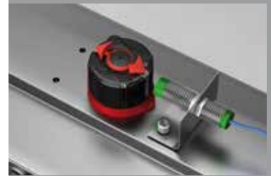
Inductive switch indicating open or closed position
